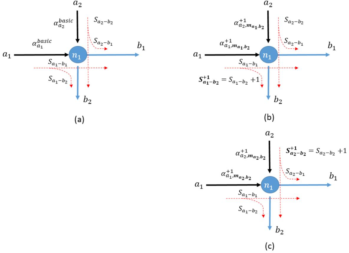
Figure 2- Computation of  $\alpha^{+1}$  for a general cross-node
