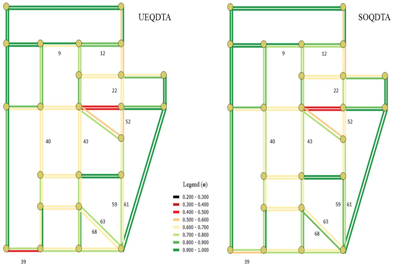
Figure 6- Link Reduction Factors under UE and SOQDTA
