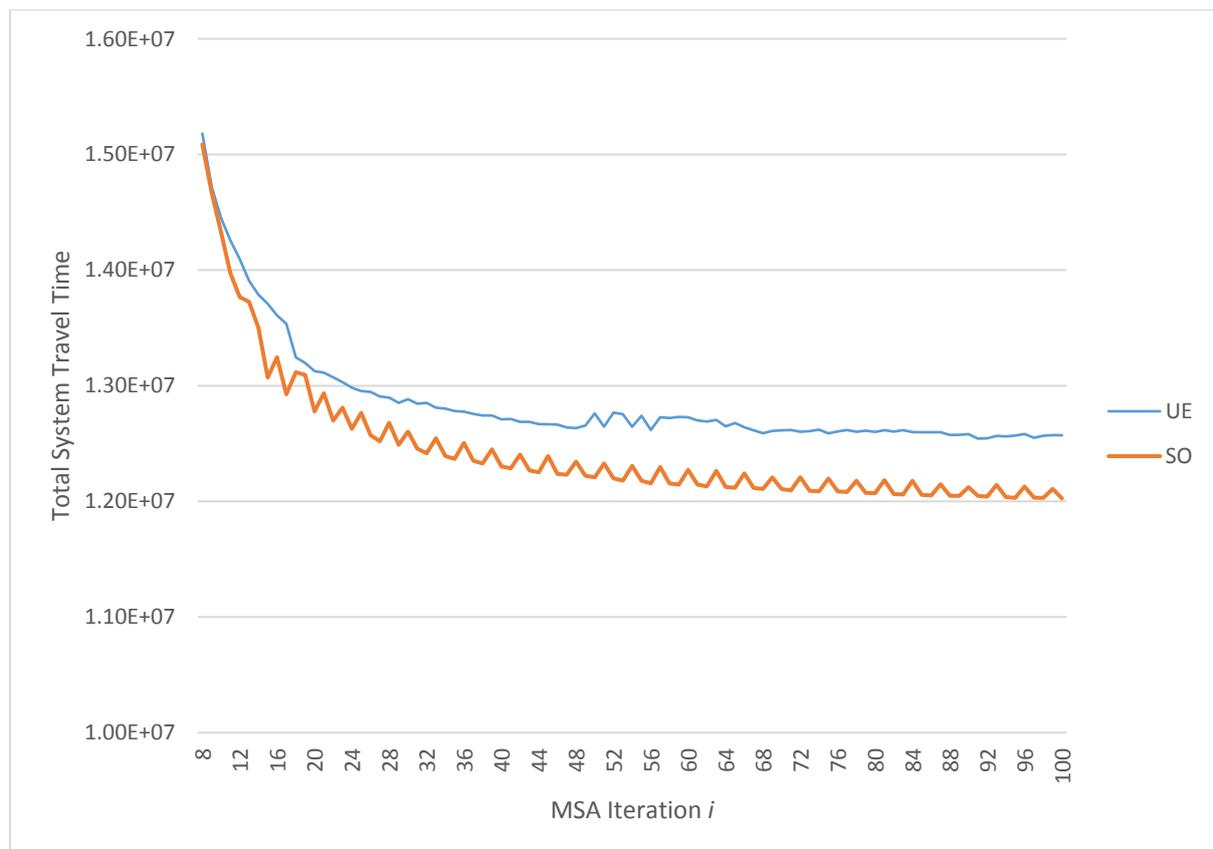
Figure 4-SOQDTA vs. UEQDTA Total System Travel Time (minutes) for the Test Network of Sioux Falls
