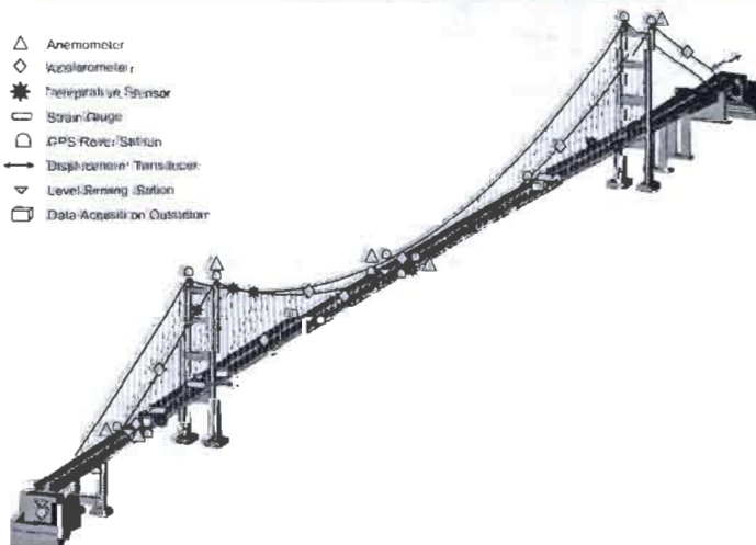
Fig. 3 Layout of the sensor and data acquisition systems (15) .
