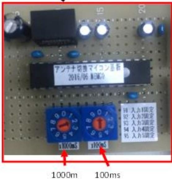
Figure 13 Inside of the antenna switch equipment
