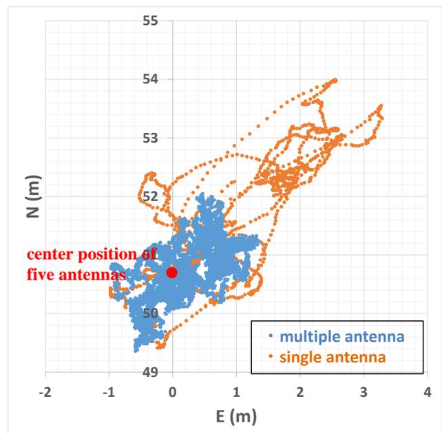
Figure 15 Comparison of horizontal position between the single antenna and the switched multiple antenna
