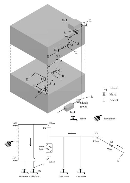
Figure 2. A simplified schematic diagram of the plumbing installation.
