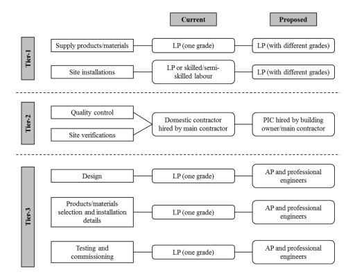
**Figure 1.** Proposed and current quality control system. Remarks: LP = licensed plumber; AP = authorized person; PIC = plumbing installation contractor.
