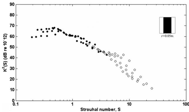
FIG. 11. Normalized 1/3 octave band results for strip spoilers in Test 2 ( $r = 0.05$  m). Values of the characteristic dimension (i.e., the total strip width)  $r$  and the drag coefficient  $C_D$ , as follows. Test 2:  $r = 0.05$  m,  $C_D = 12.0$ .
