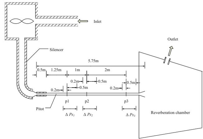
FIG. 2. (Color online) A schematic diagram of the test rig (plan view). ( $\Delta P_{S1}$ ,  $\Delta P_{S2}$ , and  $\Delta P_{S3}$ =a static pressure drop across the first spoiler, the second spoiler, and the third spoiler, respectively; p1=position at which the first test spoiler was inserted; p2=position at which the second test spoiler was inserted; and p3=position at which the third test spoiler was inserted.)
