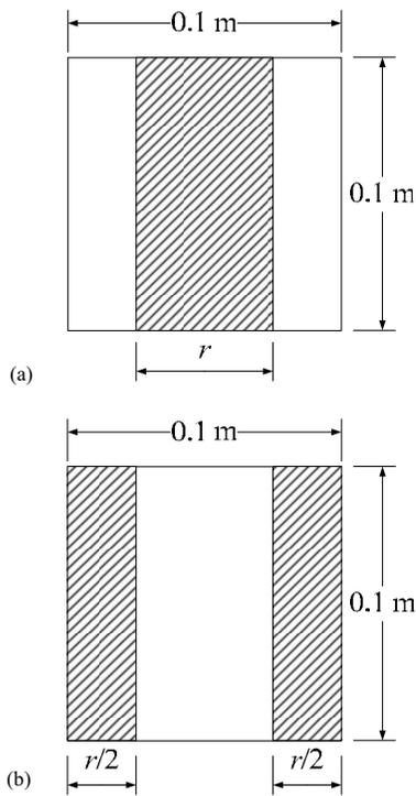
FIG. 3. Cross-section of the duct with two main types and various sizes of the flat plate strip spoilers used (shaded area). (a) Centrally placed strip spoilers;  $r=0.025, 0.05, 0.075$  m. (b) The geometries consisted of trip plates protruding symmetrically from both sides of the duct, leaving a central vertical strip of the duct open;  $r=0.025, 0.05, 0.075$  m.
