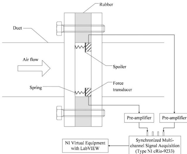
FIG. 10. A schematic diagram of the force-measuring system.
