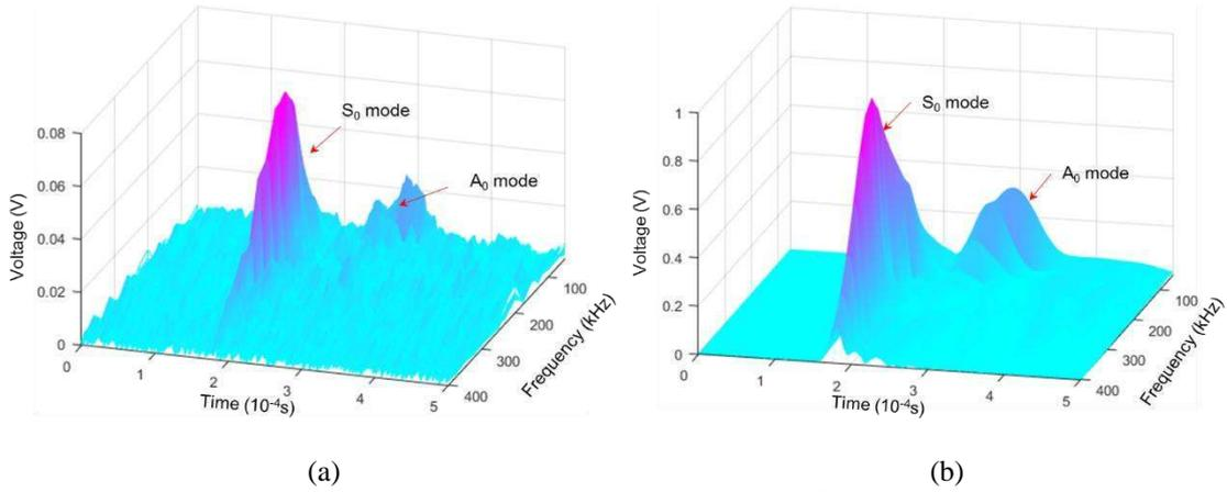
Figure 7 Magnitudes of GUVs (50kHz ~ 400kHz) acquired by (a) CB/PVDF sensor ① and (b) PZT<sub>2</sub>
