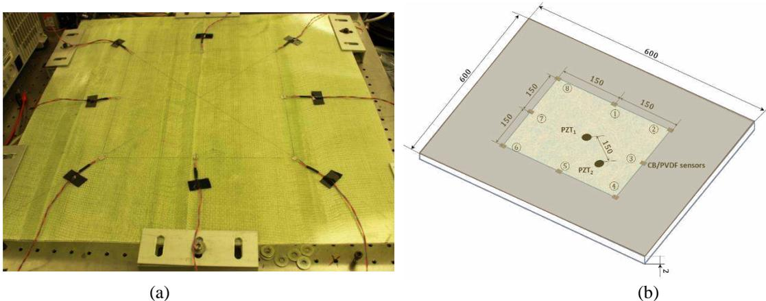
Figure 5 (a) Photographed and (b) schematic of the experimental set-up for acquisition of high-frequency
