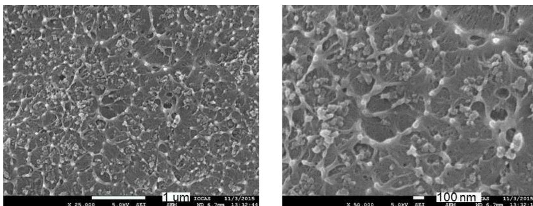
Figure 3 Nano-scalar structures of the fabricated CB/PVDF nanocomposite sensors at the CB weight ratio 6.5 wt% (right: zoomed-in SEM image of the one on left)
