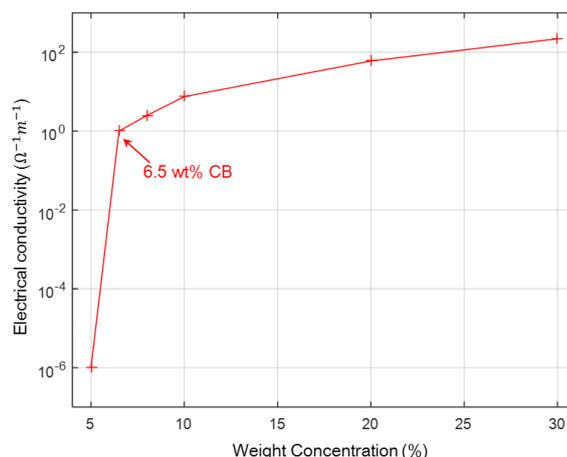
Figure 2 Average conductivity ( $\sigma$ ) of the fabricated CB/PVDF nanocomposite sensors at different CB weight ratios
