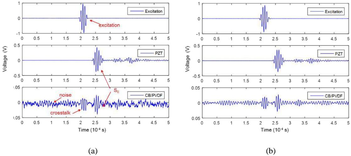
Figure 6 (a) Raw and (b) filtered signals at 150 kHz (from top to bottom: excitation signal and response signals acquired by PZT and CB/PVDF)
