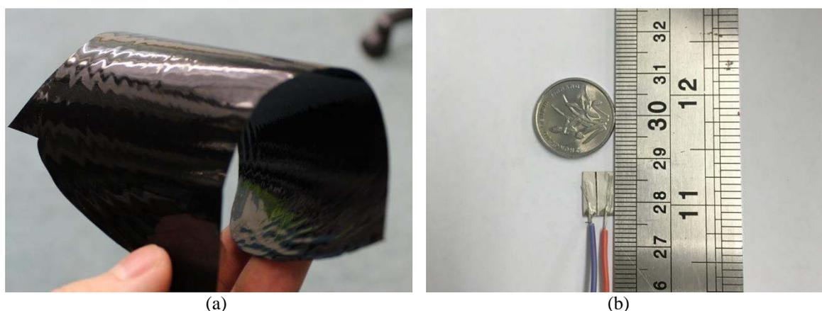
Figure 1 (a) The photographic image of the hybrid CB/PVDF and (b) a fabricated CB/PVDF nanocomposite sensor with silver pasted two electrodes
