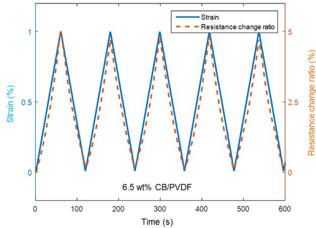
Figure 4 Electro-mechanical response of the fabricated CB/PVDF nanocomposite sensors in comparison with applied cyclic load (at percolation threshold)
