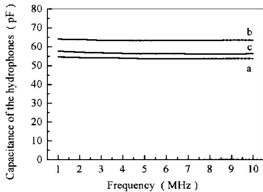
Figure 2 End-of-cable capacitance  $C$  of the hydrophones with different sensing elements as a function of frequency.
