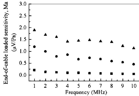
Figure 3 End-of-cable loaded sensitivity (with the amplifier)  $M_a$  of the hydrophones with different sensing elements.
