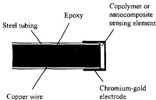
Figure 1 (a) Schematic diagram of the nanocomposite needle-type hydrophone.
