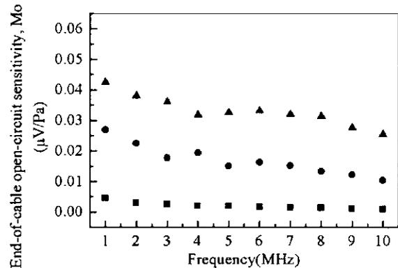
Figure 4 End-of-cable open-circuit sensitivity  $M_o$  of the hydrophones with different sensing elements.
