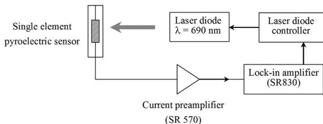
FIG. 3. Schematic setup of the measurement of current response to incident radiation.
