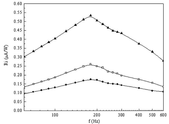
FIG. 4. Frequency dependence of  $R_i$  for lead-free BNKLBT pyroelectric sensors. Element thickness: ●—0.7 mm; □—0.5 mm; ▲—0.3 mm.
