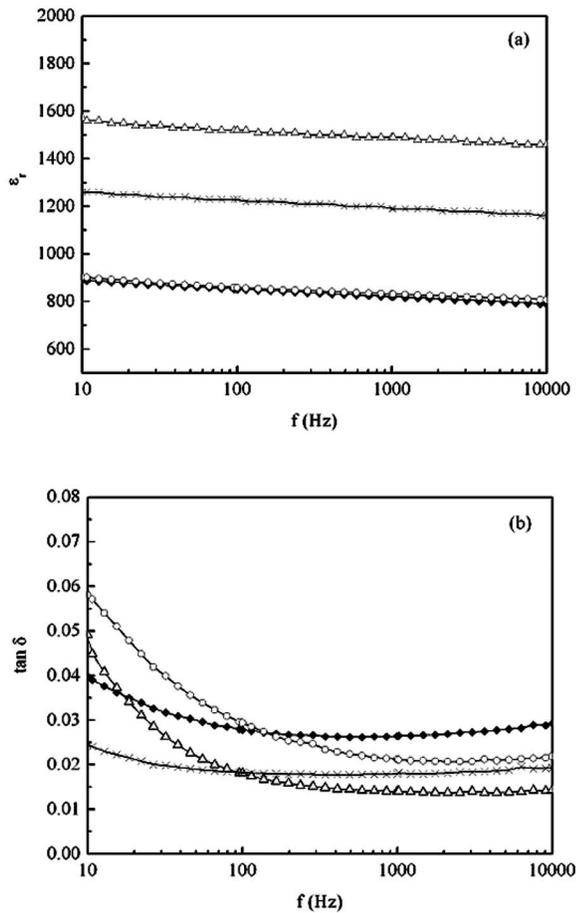
FIG. 1. Frequency dependence of (a)  $\epsilon_r$  and (b)  $\tan \delta$  for the lead-free ceramics at room temperature:  $\times$ —KNLNT;  $\triangle$ —KNLNTS;  $\blacklozenge$ —BNKBT;  $\circ$ —BNKLBT.
