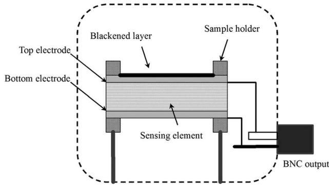
FIG. 2. Schematic diagram of the pyroelectric sensor.
