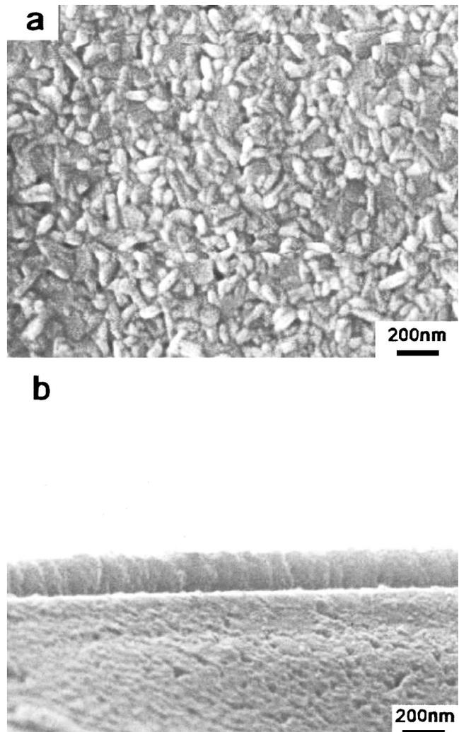
FIG. 6. The SEM images for BLT-SBTi thin film annealed at 700 °C: (a) surface morphology and (b) cross section of SEM micrograph.
