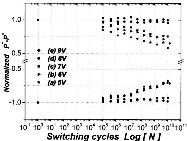
FIG. 8. Polarization degradation of 300 nm thick BLT-SBTi film at  $10^5$  Hz and 5 V (170 kV/cm); 6 V (200 kV/cm); 7 V (230 kV/cm); 8 V (270 kV/cm); and 9 V (300 kV/cm).
