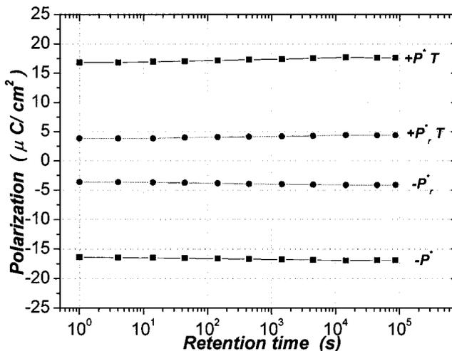
FIG. 9. The time dependence of retention properties over the range 1– $10^5$  s for BLT-SBTi thin film annealed at 700 °C.
