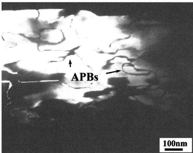
FIG. 10. Dark-field image obtained by using a superlattice diffraction spot of BLT-SBTi.
