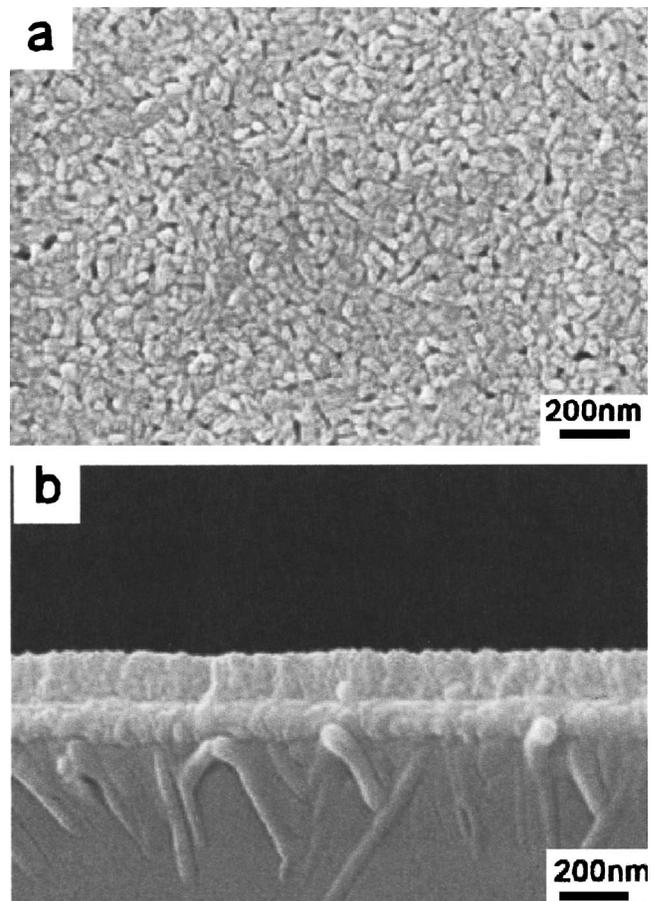
FIG. 2. The SEM images for BT-SBTi thin film annealed at 650 °C: (a) surface morphology and (b) cross section of SEM micrograph.
