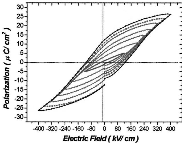
FIG. 3. The hysteresis loops for BT-SBTi thin film with different applied voltages.
