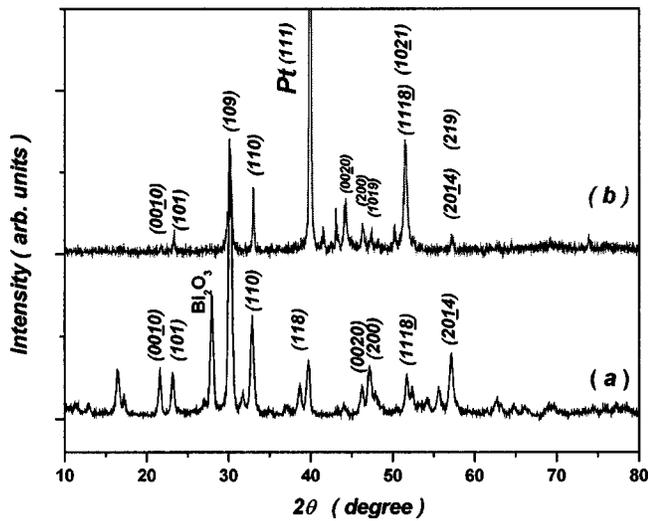
FIG. 1. The XRD pattern with Cu  $K\alpha$  radiation for BT-SBTi (a) ceramics and (b) thin film annealed at 650 °C.
