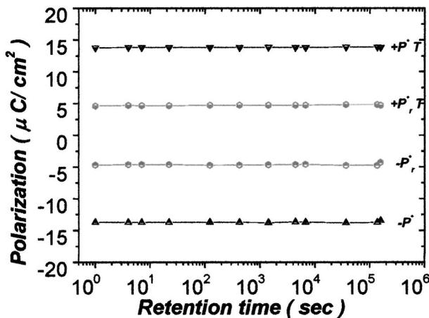
FIG. 4. The time dependence of retention properties over the range 1–10<sup>5</sup> s for BT-SBTi thin film annealed at 650 °C.
