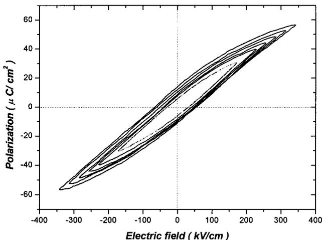
FIG. 7. The hysteresis loops for BLT-SBTi thin film with different applied voltages.
