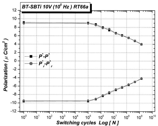
FIG. 5. The fatigue behavior with 10 V applied voltage 100 kHz for 350 nm BT-SBTi thin film annealed at 650 °C.
