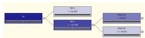
Fig.3. Regression Tree model for forecasting Mean Time between Failures (MTBF) of a D11 Dozer
