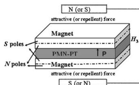
FIG. 1. Schematic diagram of NdFeB magnets/PMN-PT crystal laminate composite. The externally applied ac magnetic field ( $H_3$ ) can exert the attractive or repellent forces on the two magnet layers simultaneously.
