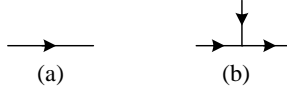
Fig. 1. Power flow sub-graphs of DISO converters with both input ports supplying power unidirectionally. (a) Type I; (b) Type II.
