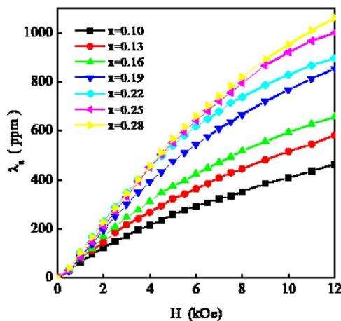
FIG. 4. (Color online) Magnetic field dependence of the magnetostriction  $\lambda_a (= \lambda_{\parallel} - \lambda_{\perp})$  for the  $\text{Tb}_x\text{Dy}_{0.7-x}\text{Pr}_{0.3}(\text{Fe}_{0.9}\text{B}_{0.1})_{1.93}$  alloys.
