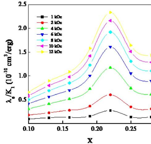
FIG. 5. (Color online) Compositional dependence of the ratio  $\lambda_a/K_1$  for the  $\text{Tb}_x\text{Dy}_{0.7-x}\text{Pr}_{0.3}(\text{Fe}_{0.9}\text{B}_{0.1})_{1.93}$  alloys.
