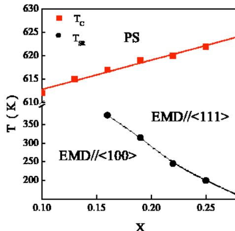
FIG. 2. (Color online) Spin configuration diagram of  $\text{Tb}_x\text{Dy}_{0.7-x}\text{Pr}_{0.3}(\text{Fe}_{0.9}\text{B}_{0.1})_{1.93}$  compounds. The squares and circles denote the Curie temperature and the spin reorientation temperature, respectively. PS represents the paramagnetic state.
