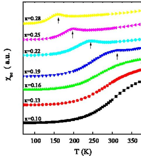
FIG. 1. (Color online) ac initial susceptibility temperature dependence  $\chi_{\text{ac}}(T)$  of the  $\text{Tb}_x\text{Dy}_{0.7-x}\text{Pr}_{0.3}(\text{Fe}_{0.9}\text{B}_{0.1})_{1.93}$  alloys. (The arrow indicates spin reorientation temperature  $T_{\text{SR}}$ .)
