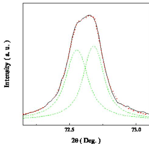
FIG. 6. (Color online) The (440) XRD line and the fitted lines of the  $\text{Tb}_{0.22}\text{Dy}_{0.48}\text{Pr}_{0.3}(\text{Fe}_{0.9}\text{B}_{0.1})_{1.93}$  alloy.
