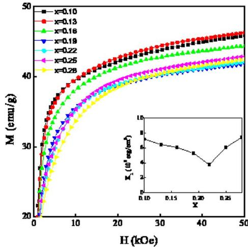
FIG. 3. (Color online) Magnetization curves and magnetocrystalline anisotropy constant  $K_1$ , at room temperature of the  $\text{Tb}_x\text{Dy}_{0.7-x}\text{Pr}_{0.3}(\text{Fe}_{0.9}\text{B}_{0.1})_{1.93}$  alloys.
