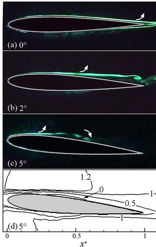
FIG. 5. Typical photographs captured in LIF flow visualization: (a)  $\alpha = 0^\circ$ , (b)  $2^\circ$ , (c)  $5^\circ$ , (d) the iso-contours of PIV-measured  $\bar{U}^*$  ( $\alpha = 5^\circ$ ).  $Re_c = 2.0 \times 10^4$ . Symbols  $\nearrow$  and  $\searrow$  indicates the occurrence of flow separation and reattachment, respectively.
