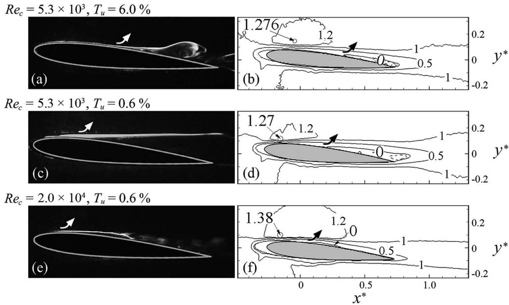
FIG. 16. Effect of  $Re_c$  or  $T_u$  on the flow separation point at  $\alpha = 5^\circ$ . Left column: photographs of instantaneous flow structure captured from LIF flow visualization; right column: iso-contours of PIV-measured time-averaged streamwise velocity  $\bar{U}^*$ . Symbol  $\blacktriangleright$  indicates the occurrence of flow separation.
