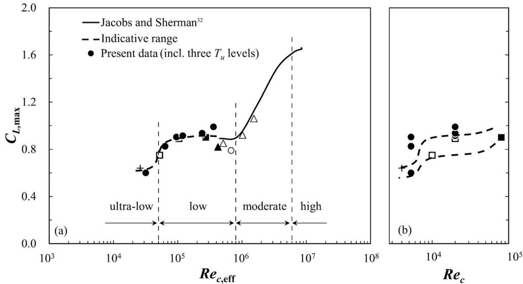
FIG. 15. Dependence of the maximum lift coefficient  $C_{L,max}$  on (a) effective Reynolds number  $Re_{c,eff}$ , (b) test Reynolds number  $Re_c$ : + Sunada *et al.*<sup>25</sup>; ■ Chen and Choa<sup>35</sup>; □ Cleaver *et al.*<sup>26</sup>; ○ Grager *et al.*<sup>36</sup>; ◆ Lee and Gerontakos<sup>37</sup>; ▲ Wong and Kontis<sup>38</sup>; △ Sant and Ayuso.<sup>39</sup>
