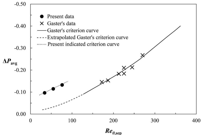
FIG. 21. Relation between  $Re_{\theta,sep}$  and  $\Delta P_{avg}$  at bursting.
