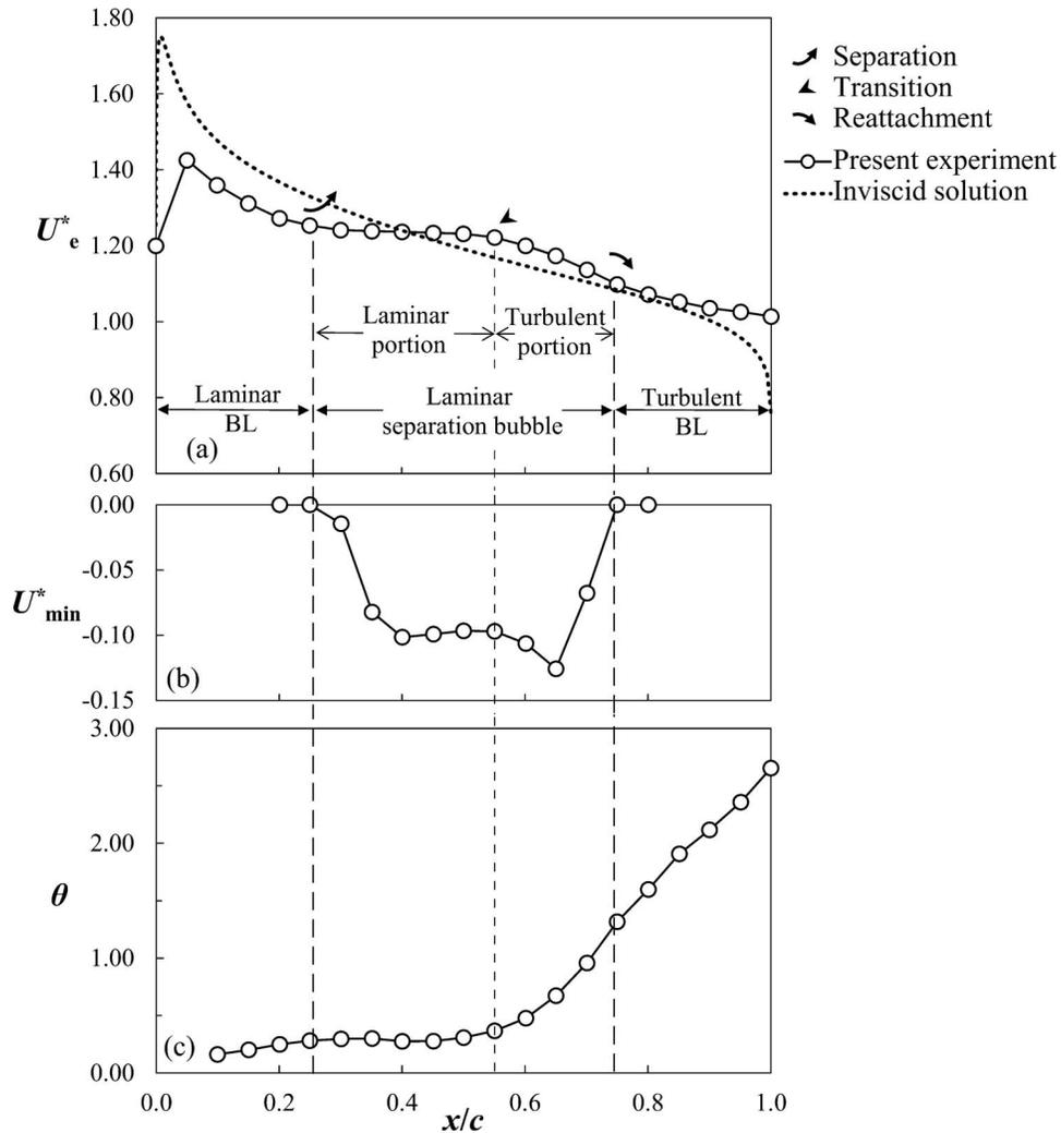
FIG. 19. (a) Normalized boundary layer edge velocity  $U_e^*$ , (b) normalized minimum velocity  $U_{\min}^*$ , and (c) momentum thickness  $\theta$  of the boundary layer at  $\alpha = 5^\circ$ .  $Re_c = 2.0 \times 10^4$ .
