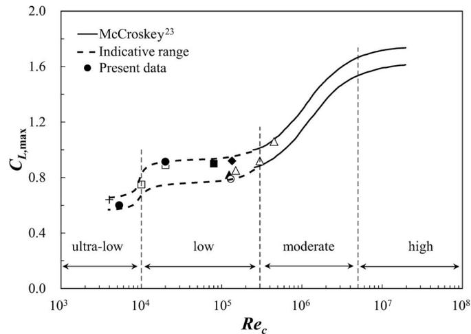
FIG. 7. Dependence of  $C_{L,max}$  on  $Re_c$  of NACA 0012 airfoil: + Sunada *et al.*<sup>25</sup>; ■ Chen and Choa<sup>35</sup>; □ Cleaver *et al.*<sup>26</sup>; ○ Grager *et al.*<sup>36</sup>; ◆ Lee and Gerontakos<sup>37</sup>; ▲ Wong and Kontis<sup>38</sup>; △ Sant and Ayuso.<sup>39</sup>
