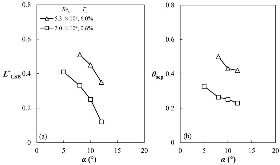
FIG. 20. Dependence of the laminar separation bubble (LSB) on  $\alpha$ : (a) normalized bubble length  $L^*_{LSB}$  and (b) momentum thickness  $\theta_{sep}$  of the boundary layer at separation.
