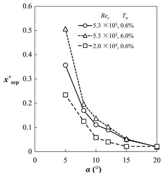
FIG. 17. Dependence of the flow separation point  $x_{sep}^*$  on  $\alpha$ .
