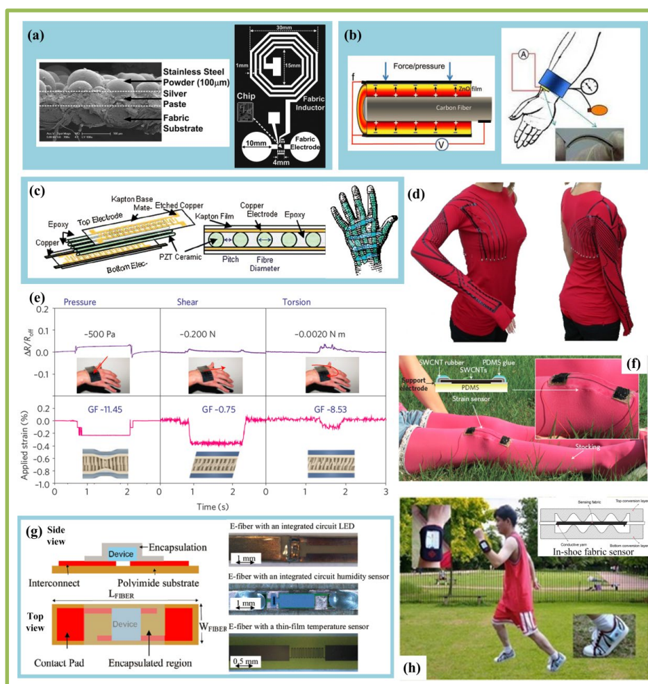
Figure 8. Fiber-based sensors: (a) Fabric bio-potential electrode and its SEM photo, [150] (b) Pulse-driven fiber nanogenerator by ZnO thin films grown around a carbon fiber as a strain sensor, [6a] (c) Vibration sensor arrays of piezoelectric fibers in gloves for detection and suppression of Parkinson's tremor in the hand, [151] (d) Carbon loaded elastomer sensorized garment for kinesthetic monitoring, (e) Strain-gauge sensor based on the reversible interlocking of Pt-coated polymer nanofibres, [142k] (f) Carbon nanotube strain sensor for human motion detection, [20c] (g) Woven electronic fibers with sensing and display functions, [5b] (h) In-shoe plantar pressure monitoring in daily activities by fabric pressure sensors. [142i]
