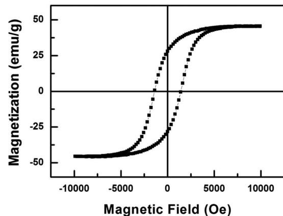
FIG. 5. Magnetization hysteresis loop for the CFO/P(VDF-TrFE) nanocomposites.
