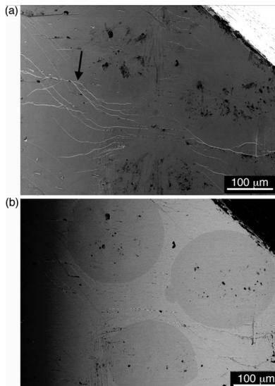
FIG. 3. (a) SEM image showing shear bands near intermetallic particles in the  $Zr_{55.0}Cu_{29.0}Ni_{8.0}Al_{8.0}$  intermetallic/BMG composite, and (b) backscattered electron image (BSE) showing the position of intermetallic spheres in the same sample.
