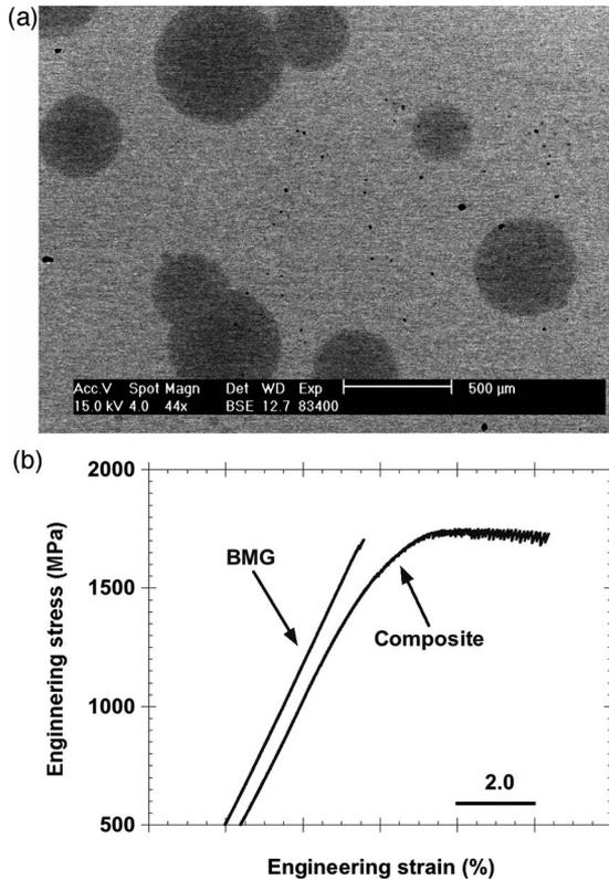
FIG. 1. (a) Backscattered electron image, and (b) compressive engineering stress-strain curve for  $Zr_{55.0}Cu_{29.0}Ni_{8.0}Al_{8.0}$  intermetallic/BMG composite with a diameter of 10 mm. For comparison, a monolithic BMG with same composition is also included.
