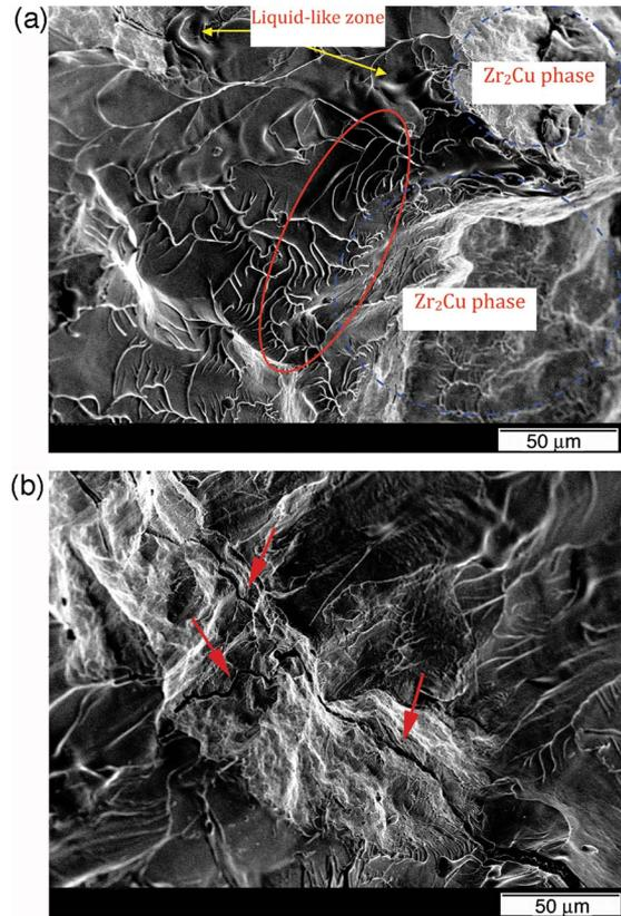
FIG. 2. (Color online) SEM fracture surface of the  $Zr_{55.0}Cu_{29.0}Ni_{8.0}Al_{8.0}$  intermetallic/BMG composite: (a) Veinlike patterns in the glassy matrix, and (b) cracks in the intermetallic phase.
