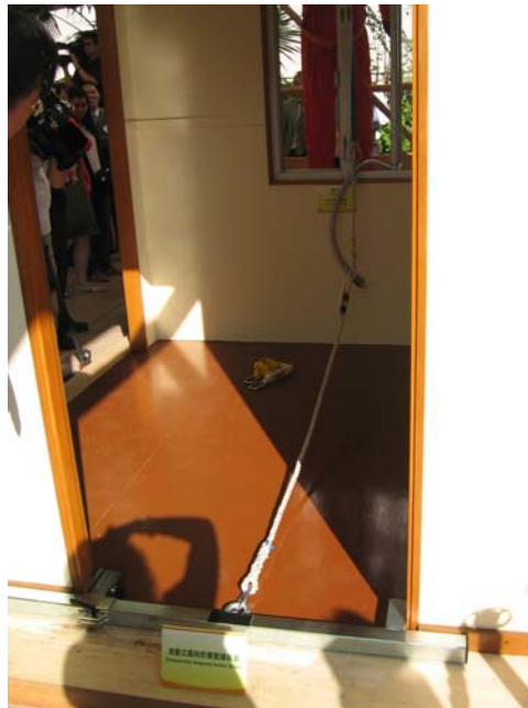
Figure 4.4 A temporary transportable anchor device against a door frame – demonstration from an OSHC seminar
