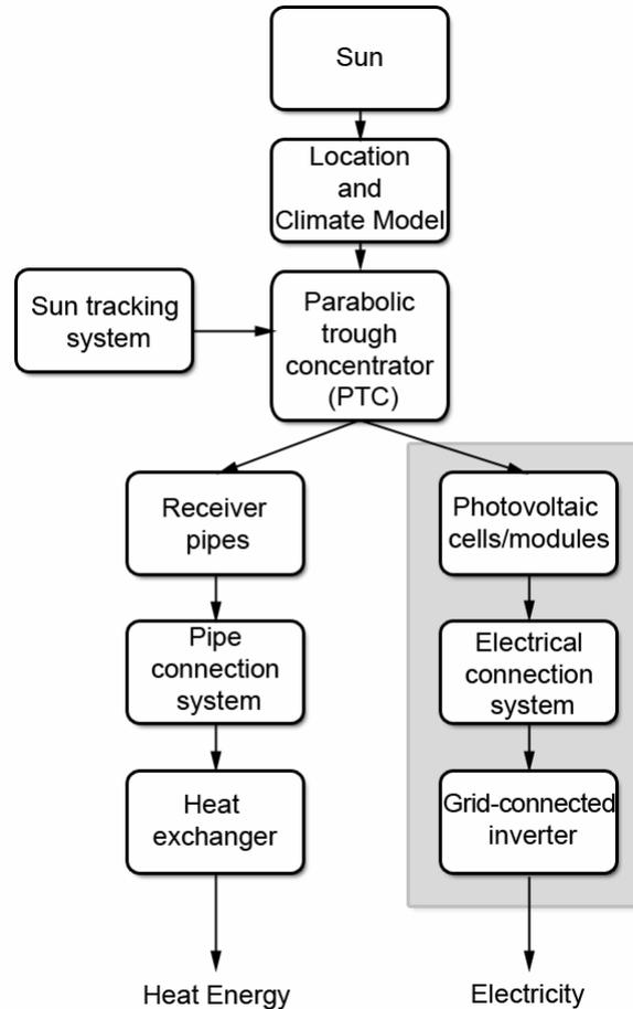
Figure 2 Structure of hybrid PTC simulation software
