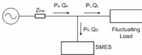
Fig. 4. Schematic diagram to compensate for fluctuating load
