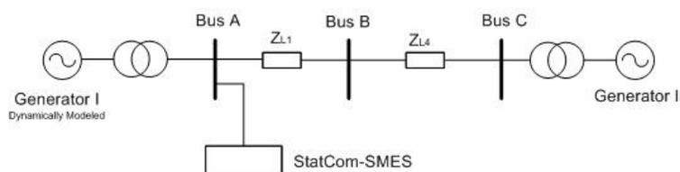
Fig. 3. Schematic improving FACTS performances using SMES
