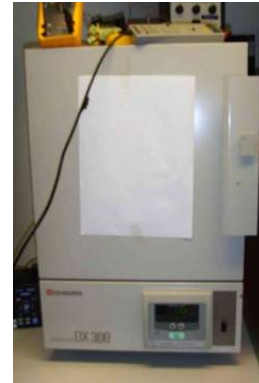
Fig 10: Thermal chamber used for the endurance test
