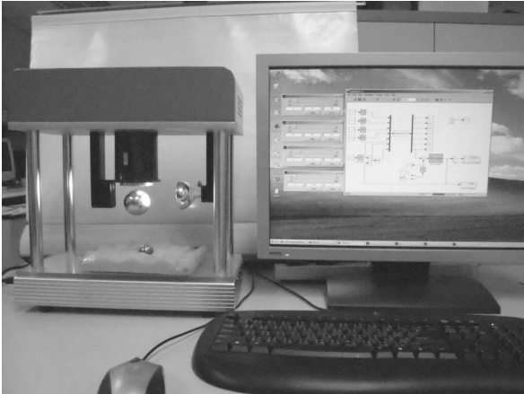
Fig. 1. Experimental setup of the magnetic levitation system
