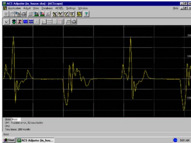
Fig. 7: Dynamic error position (y-axis: 50 counts per division).
