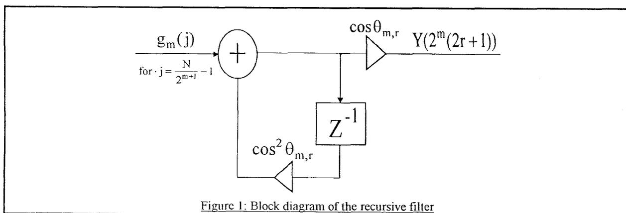
Figure 1: Block diagram of the recursive filter
