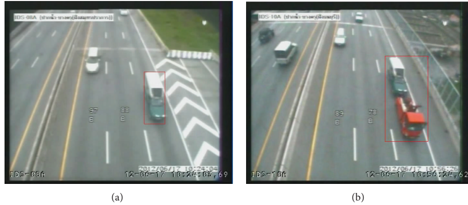
FIGURE 8: Real-world case study #2: (a) incident vehicle passes the upstream detector; (b) incident vehicle and truck passes through the downstream detector.
