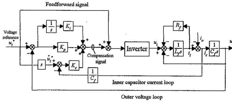
Fig.4. Multiple-feedback-loop control scheme to obtain example patterns under linear loading conditions
