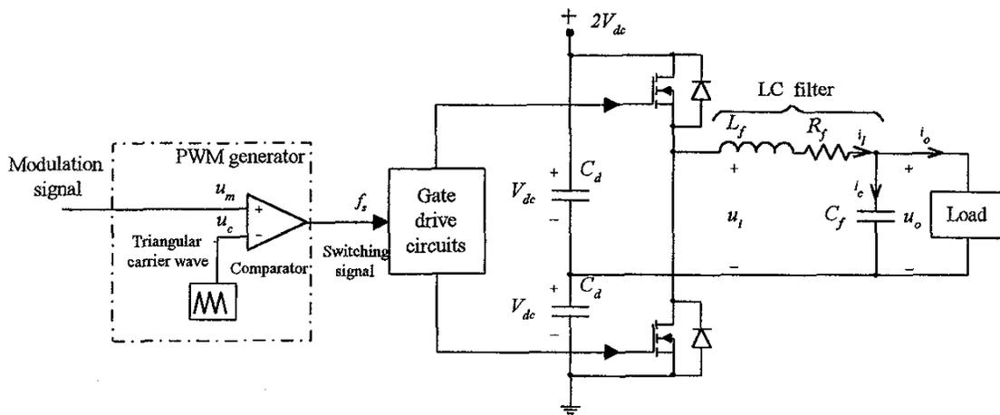
Fig. 1. Single-phase UPS inverter system
