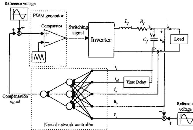
Fig.6. Proposed neural network control scheme for UPS inverter
