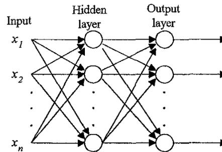
Fig. 3. Structure of a two layer feedforward neural network
