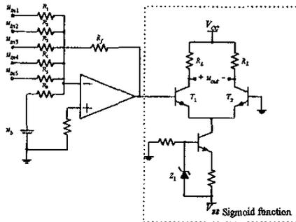
Fig.7. An analog circuit realization of a neuron
