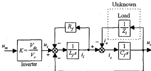
Fig. 2. Linear model of UPS inverter
