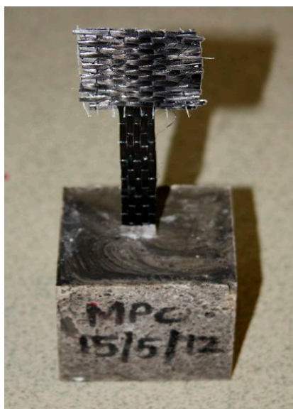
Figure 2. Pullout test specimen.
