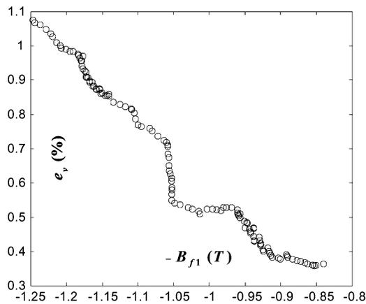
Fig. 6. Computed Pareto front by Emigration Pareto Evolutionary Algorithm (EPEA) for the 400-MW, 44-pole hydrogenerator.
