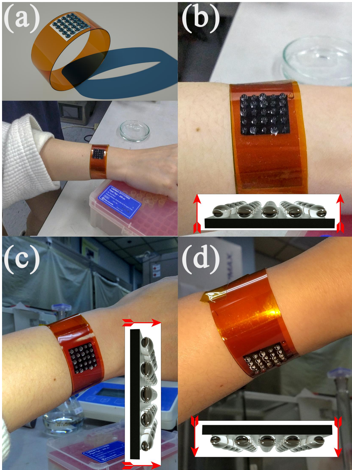
Figure 3 Demonstration of the wearable water-capturing device. (a) A wristband type water capture device worn on the human arm, with captured water when facing up (b), sideways (c), and down (d).
