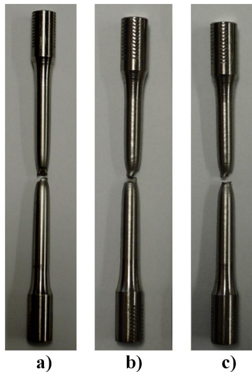
Fig. 9. The fractured tensile test specimens at strain rates of: a) 0.001 \text{ s}^{-1} ; b) 0.005 \text{ s}^{-1} and c) 0.01 \text{ s}^{-1} .
