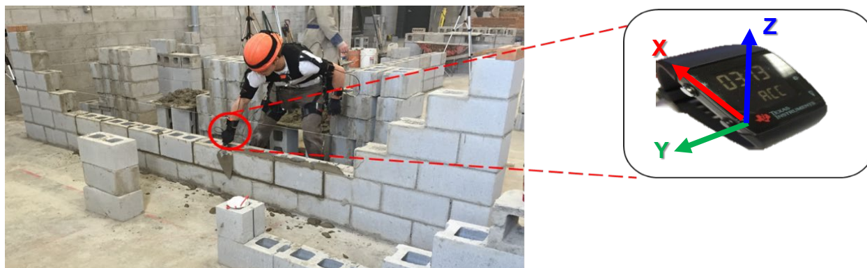
Figure 2. Test setup and the subject's performance with detail of wearable device
