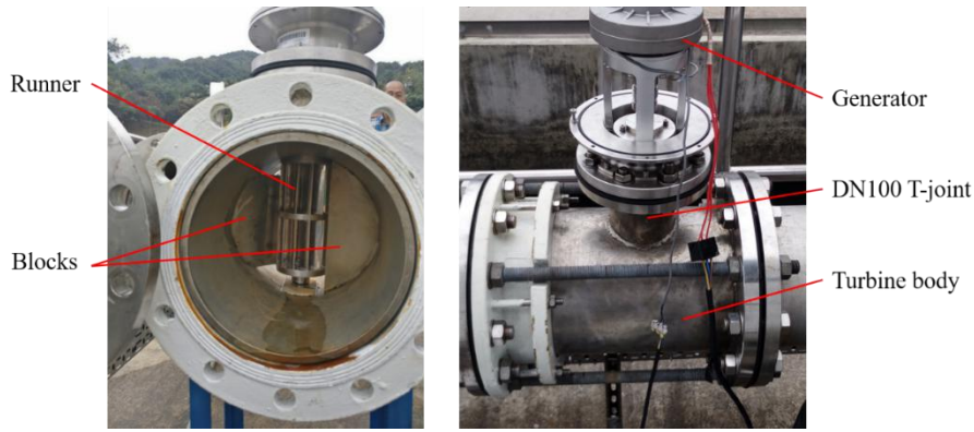
Fig. 1 Prototype of the previously developed inline cross-flow turbine
