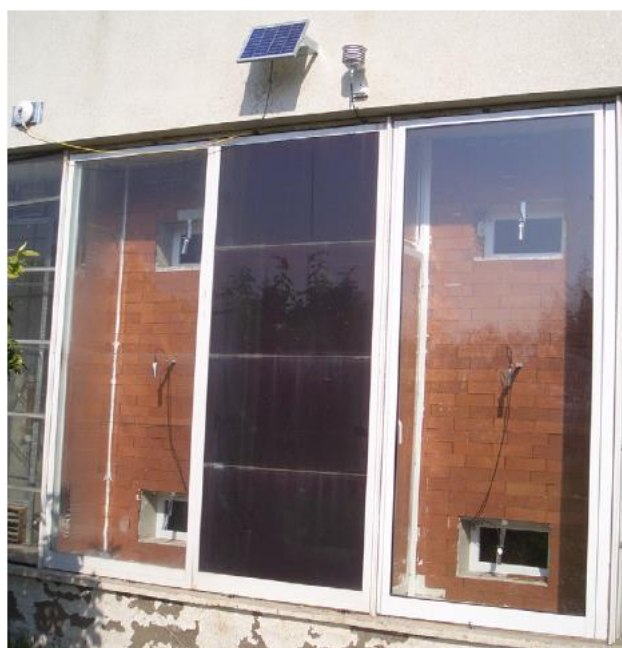
Left: single-glass wall; Middle: PV-wall; Right: Double-glass-wall
