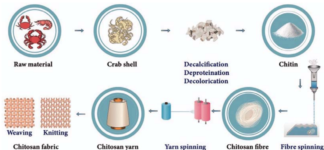
Figure 1. Procedures of raw materials to fabric in the chitosan textile industry.
