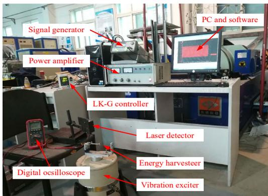
Fig. 8 The experimental equipment
