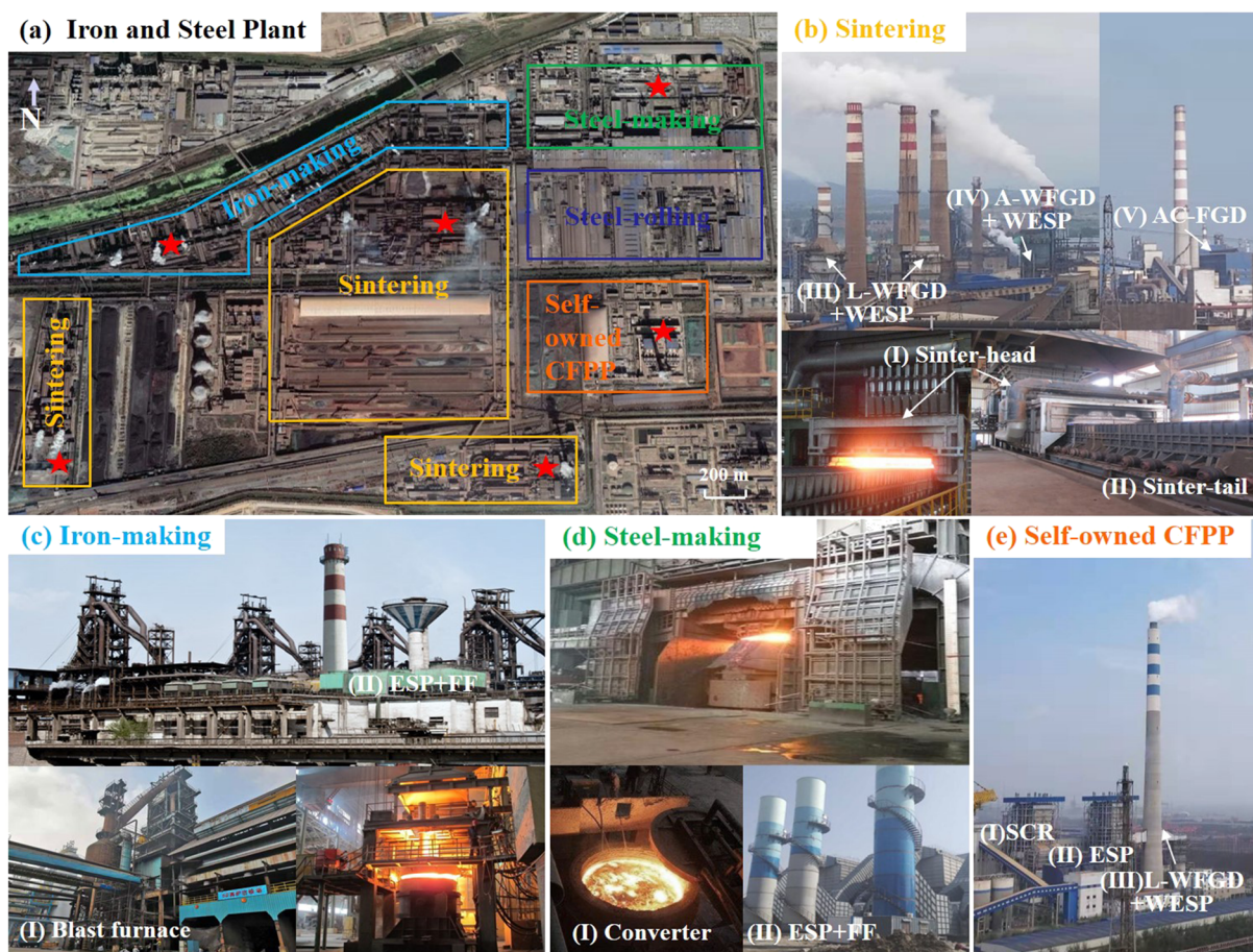
Figure 1. (a) Location of the sampling sites in the tested iron and steel plants; (b) sintering process: (I) the head of sintering machine (sinter head), (II) the tail of sintering machine (sinter tail), (III) lime-gypsum wet flue gas desulfurization (L-WFGD), (IV) ammonia wet flue gas desulfurization (A-WFGD), and (V) activated coke dry flue gas desulfurization (AC-FGD); (c) ironmaking process: (I) the blast furnace and (II) electrostatic precipitator + fabric filter (ESP + FF); (d) steelmaking process: (I) the converter and (II) ESP + FF; and (e) self-owned CFPP: (I) selective catalytic reduction (SCR), (II) ESP, and (III) L-WFGD.
