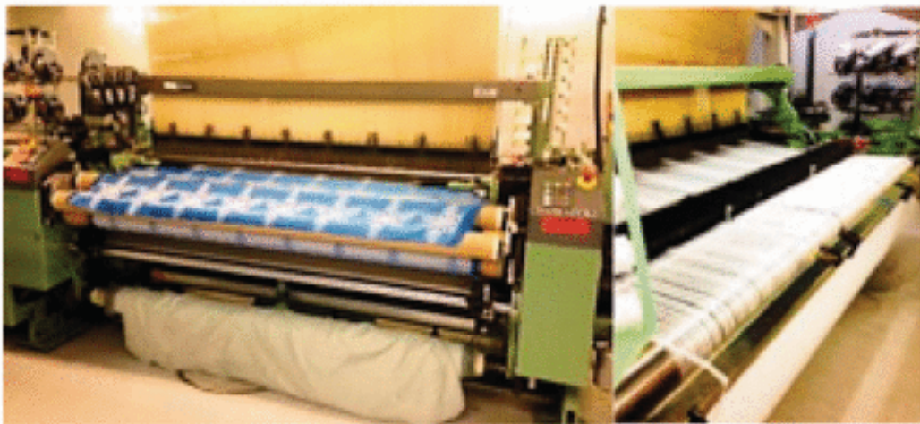
Figure 2. STAUBLI F-69680 high-speed jacquard machine.
