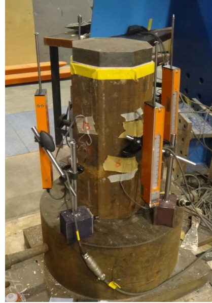
(b) Octagonal confined specimen
