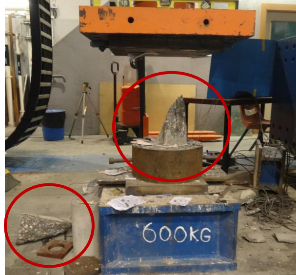
(b) Exploded high-strength concrete core
