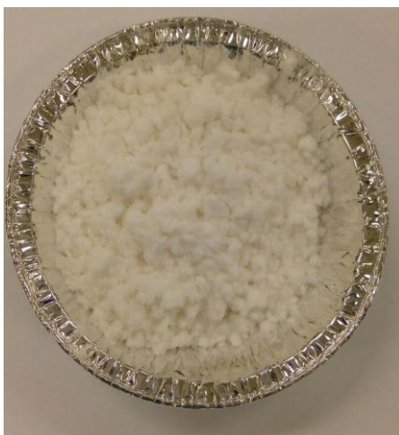
3 4 Figure 1. BHETA Additive after Aminolysis
