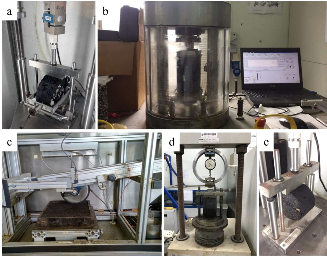
FIGURE 2 Conducted tests: (a) ITSM; (b) SPT; (c) LWT; (d) ITS; (e) ITFT
