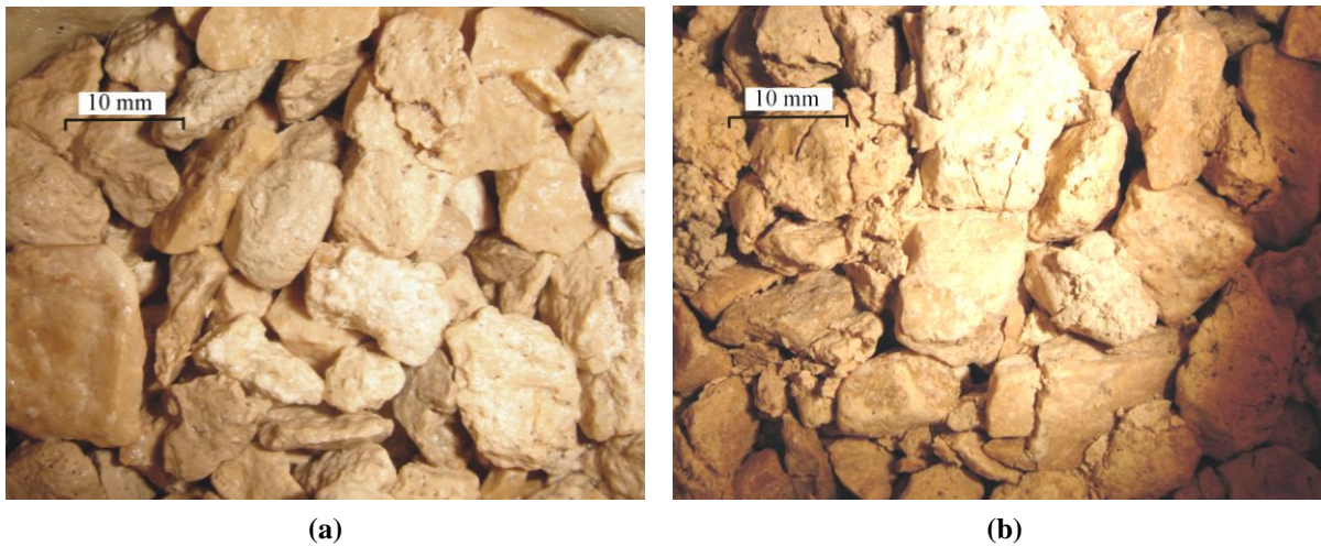
Fig. 2. Photographs of a tested sample: (a) before testing, and (b) after testing under constant p' = 400 kPa.
