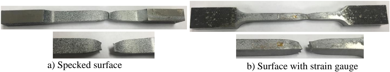
Figure 9: Typical failure mode of a S690 steel coupon
