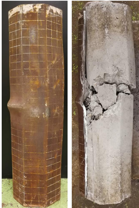
Figure 10. Failure mode of concrete core of specimens S30O-2
