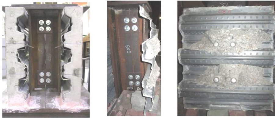
Figure 2: Typical concrete conical failure in shear connections with composite slabs
