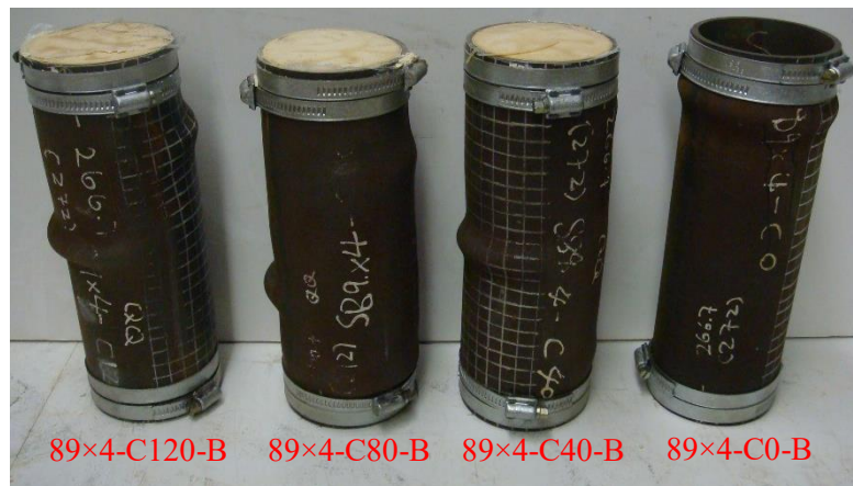
Figure 3: Failure modes of CFHSS circular stub column specimens for Series 89×4
