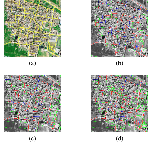
Fig. 10. Comparison of the results of different road extraction strategies on the Xuzhou test area: (a) ground truth; (b) EM results; (c) linear-ness filter results; (d) fusion result. TP, FP, and FN are shown in red, green, and blue, respectively.
