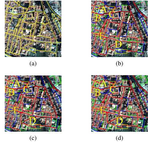
Fig. 9. Comparison results of different road extraction strategies on the Pavia test area: (a) ground truth; (b) EM result; (c) linear-ness filter result; (d) information fusion result. TP, FP, and FN are shown in red, green, and blue, respectively.
