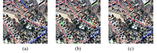
Fig. 8. (a), (b), and (c) show the information fusion results of rule set I, rule set II, and rule set III, respectively. TP, FP, and FN are shown in red, green, and blue, respectively.
