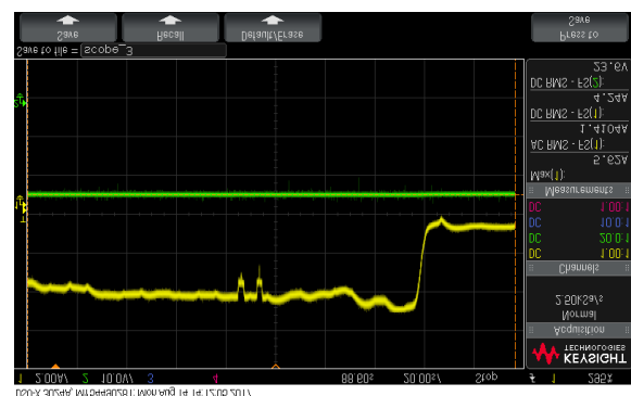
Fig 9: Oscilloscope showing the Current and voltage to the battery of the 4 solar panels connected in series. (top: current 2A/div, bottom 10V/div)
