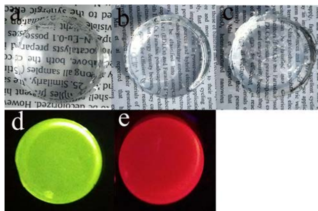
Fig. 1 Digital photos of the hydrogels: PNIPAM (a), PNIPAM- \text{Tb}(\text{DPA})_3 (b) and PNIPAM- \text{Eu}(\text{DPA})_3 (c) under daylight, and PNIPAM- \text{Tb}(\text{DPA})_3 (d) and PNIPAM- \text{Eu}(\text{DPA})_3 (e) under UV light (254 nm, 6 W)
